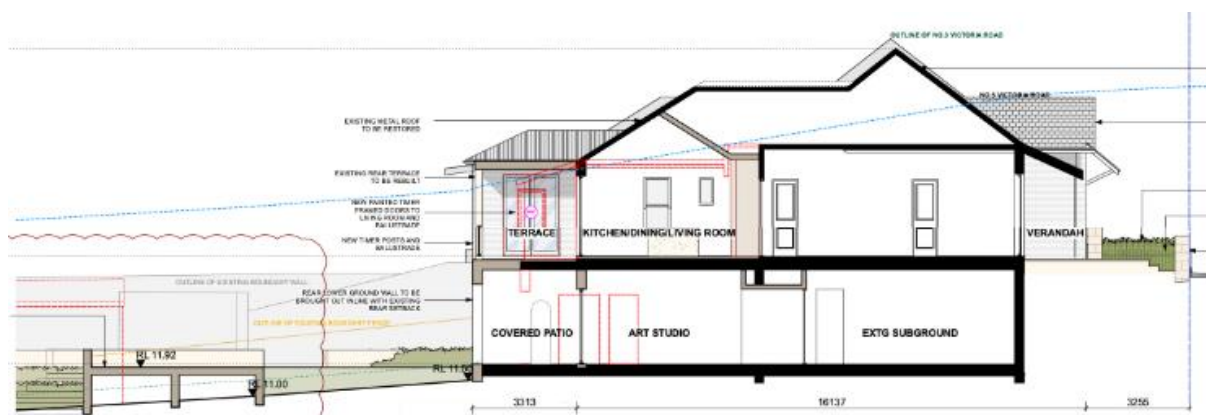
Figure 37: Proposed long section – Dwelling 1 (ground floor) and Dwelling 3 (lower ground floor)
